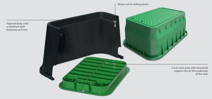
One piece molded from polyolefins (polyethylene and polypropylene). Designations for irrigation control valve and reclaimed water.
