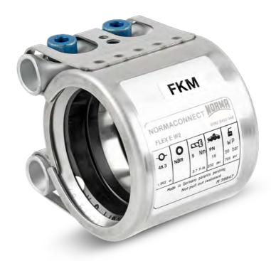
The NORMACONNECT® FGR with the FKM sleeve couples pipes with OD 33.7 - 168.3 mm, and temperatures ranging -10 °C to +150 °C or up to +180 °C for liquid media.
